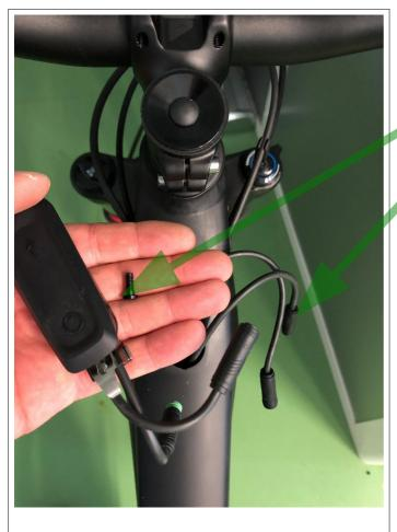
Remove the screw and disconnect the connectors by gently pulling them. Replace the TCU and connect the ADAMO19 cables paying close attention to the polarization pins and inserting them perfectly straight.
