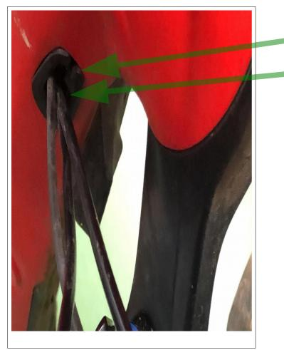
In the TL2018 unscrew the screw, remove the plastic, then cut just enough to create space so that the additional cable is just right. On other bikes, drill the frame at that point or run the cable outside.
