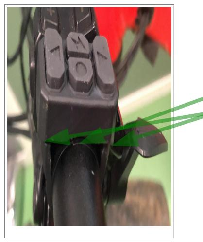
Make a round of electrician's tape where the remote will be placed.
