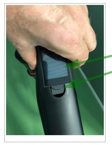
After having made all the cables enter the tube, insert ADAMO19 inclined, making sure that the rectangular tongue will enter the tube, while the round one must remain external. Upon insertion, it will be slightly forced, but still use the utmost delicacy. Help yourself with a thin metal strip.
