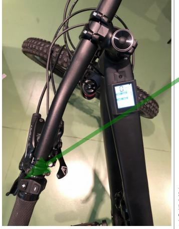
When everything is finished, keep the TURBO button pressed for a long time to turn on the bike and check that the display is on. Press the TURBO button again for a long time until the bike is switched off.
