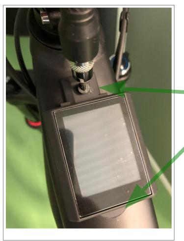
Tighten again taking care not to overtighten the screw as it is very delicate and could break. Note that the round tongue of ADAMO19 is outside the tube.
