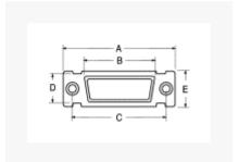
TENS. LAVORO:300 V CORRENTE MAX:5 A TEMP. LAV.:-20°C ÷ +80°C CONTATTI:rame ISOLAMENTO:poliestere COPERCHI:5/6600 DISTANZIATORI:5/6700 PER CONN.:5/6120-5/6140
