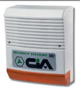
Operating test at battery connection. Power supply and lamp protection fuse. Activation on power less. Antiopening and antitearing protection tampers. Enforced ABS made box, with LURAN made flasher . Internal protection panel made in steel sheet coated with epoxy powder. NOX steel screws. Internal space for 12V 2Ah battery (not included). According to the 2° level of CEI 79-2 standard. 2nd level IMQ-Allarme certified.
