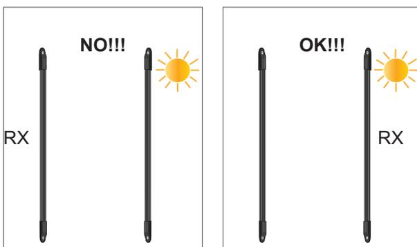
It is important that the receiver and transmitter are aligned for the best reception of the signal. When the alignment is not good, the barrier can't work properly. Pay attention for the receiver of the direct sun-light.
